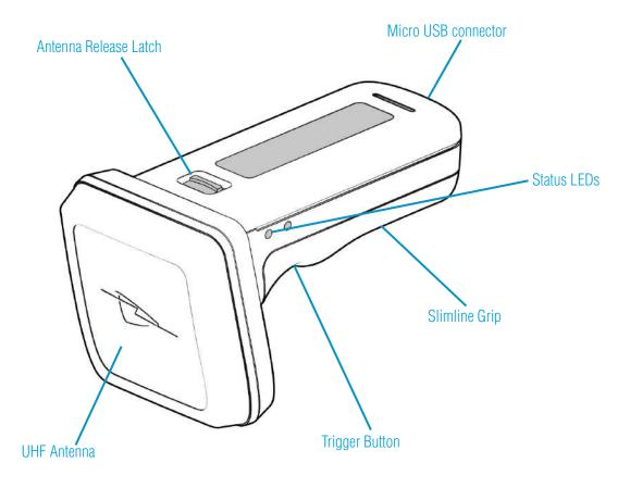
Figure 2: Parts of the 1128 UHF Reader
