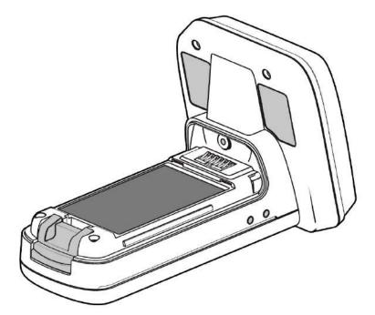
Figure 8: Battery in position
