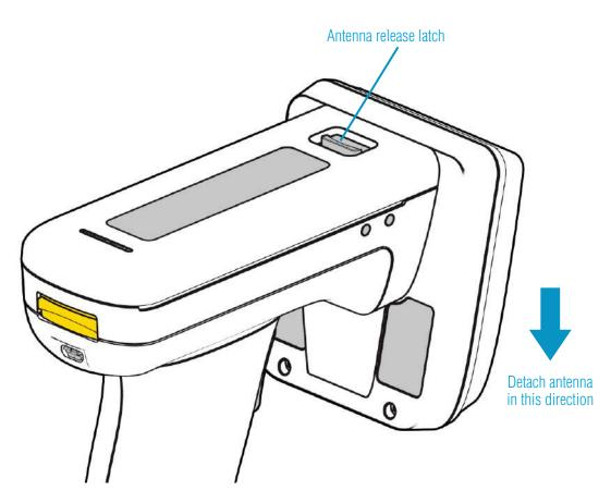
Figure 12: Antenna release latch location
