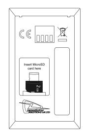
Figure 29: Micro SD Card Insertion and Removal
