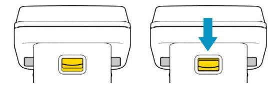
Figure 11: Antenna release latch operation
