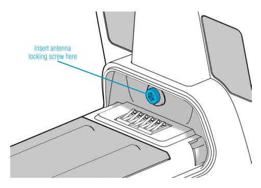
Figure 13: Antenna locking screw location
