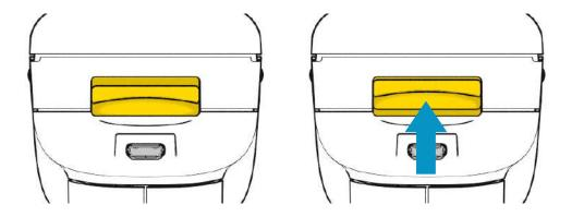
Figure 4: Handle release latch operation
