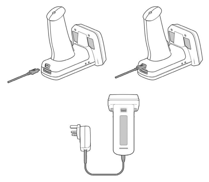
Figure 14: Attaching the Micro USB cable
